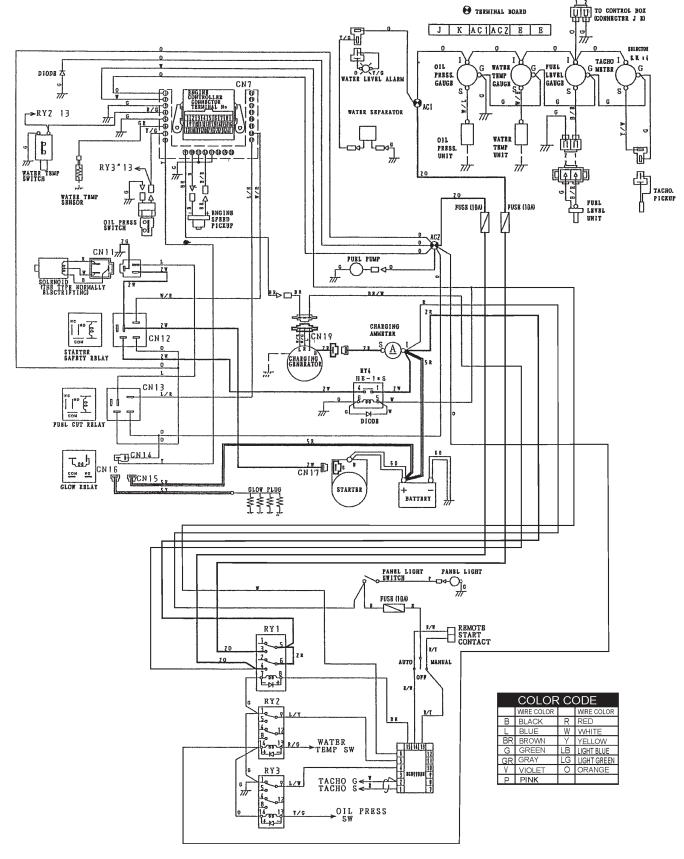
Figure 49. Engine Wiring Diagram
